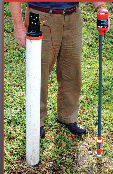
Potential meter with optional 30" electrode extension Item #16203
