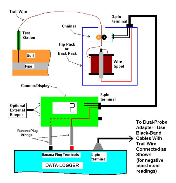
Figure 2: Counter/Display Unit Mounted Directly on Data-Logger -Connections for Manual Triggering of Readings Using Data-Probe Push-Buttons
