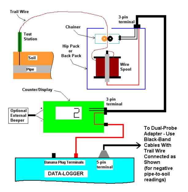
Figure 1: Counter/Display Unit Mounted on Tray – Connections for Manual Triggering of Readings Using Data-Probe Push-Buttons
