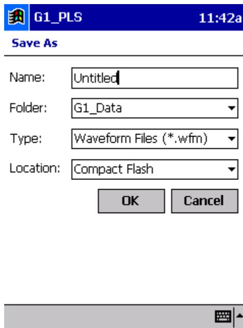
You are being asked here to establish a file in which the waveform data will be stored (saved). The name of this file will be the name you type into the “Name” box on the above screen. For ease of future retrieval when you uploaded your survey data to the Data Management software package (ProActive) [see Section VI], it is recommended that you use the same name
