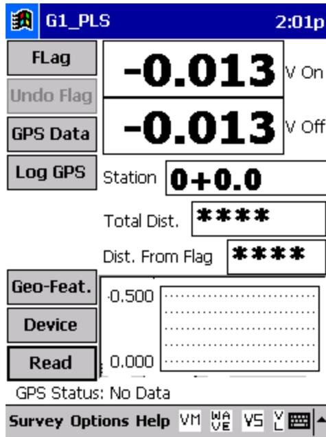
As voltages are recorded by the data-logger (by either tapping on the “Read button on the Survey screen or by pressing the appropriate cane push button, the “Total Distance” (total distance from the start of the survey) parameter will increase in increments of 2.5 feet, or whatever the “feet per reading” value was that was entered back at Step 19.
