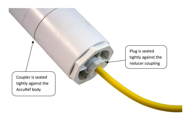
After the glue cures, the Permanent Electrode with spliced wire is ready for installation.
